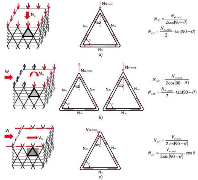
Figure 3. Diagrid module: (a) effect of gravity load, (b) effect of overturning moment and (c) effect of shear force.
