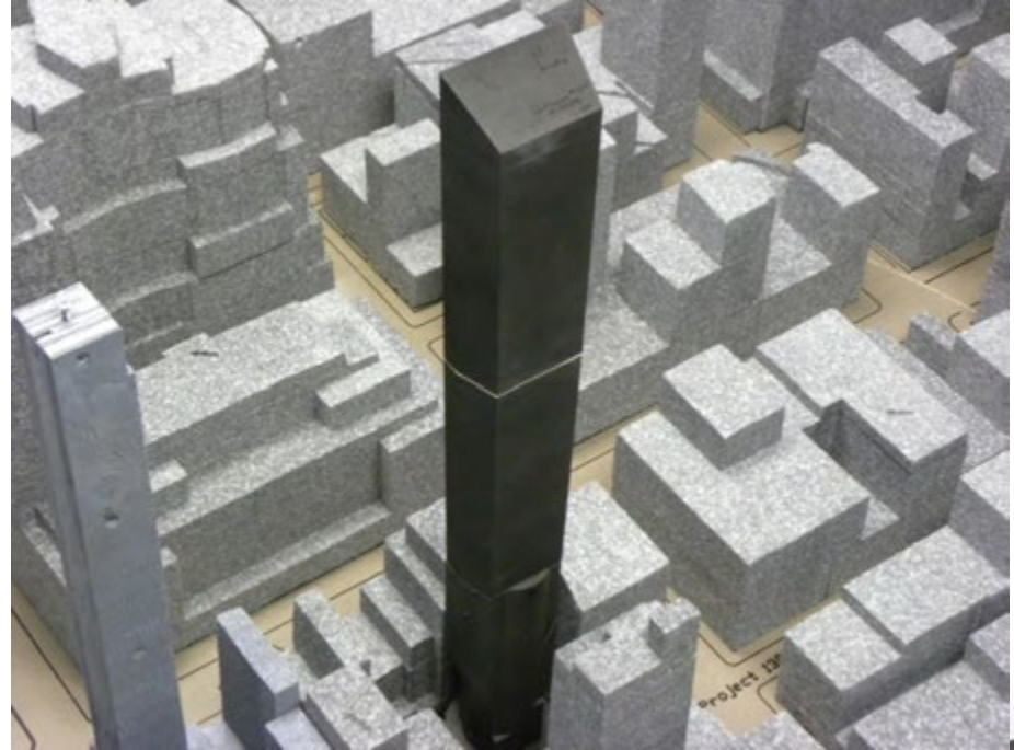
Wind Tunnel Test at RWDI
