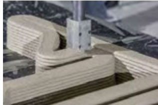
Testing 3-D printed concrete for Project Milestone, an initiative with the goal of building 3-D printed houses starting in 2019 (photo courtesy of 3dprintedhouse.nl)
