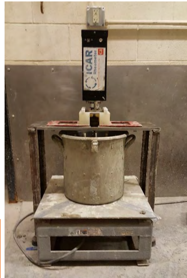
Set-up of ICAR rheometer and bucket with vibration table
