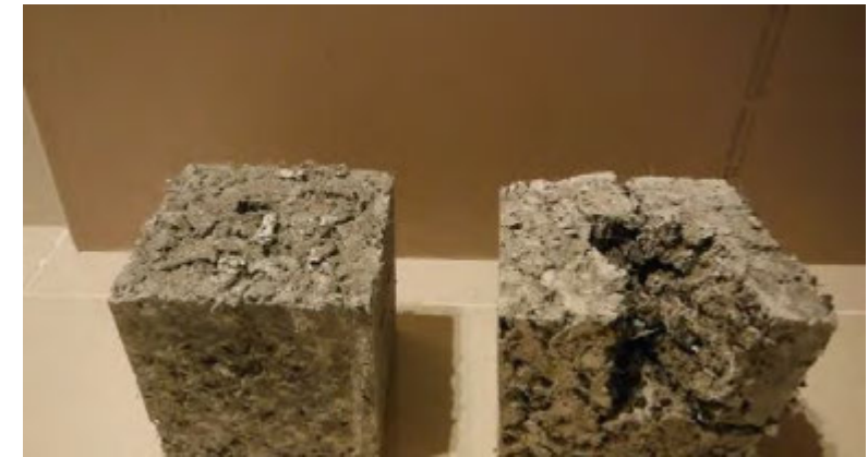
Ballistic-proof foam concrete composite
