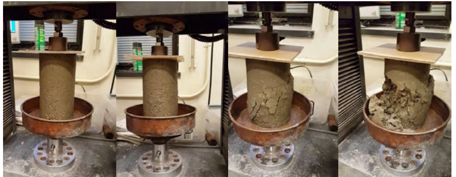
Demonstration of compressive loading of fresh, no-slump concrete 21
