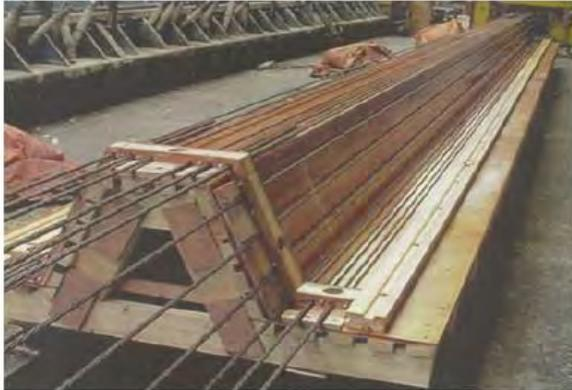
. Prestressing strands and formwork used for production of SCFRC sheet piles (Walraven 2007)
