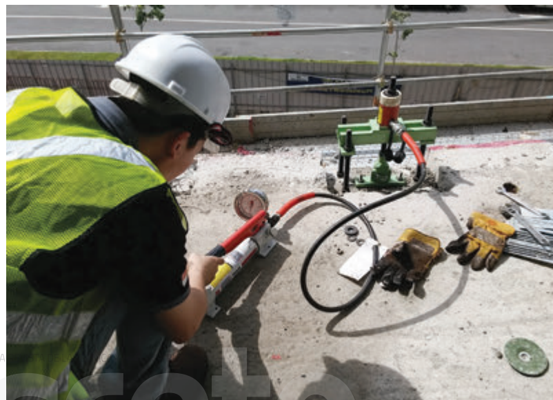
↑ Ensayo de pull-out ASTM C900. © CONQUALITYTIPS
