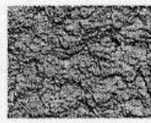
CSP 7 (heavy abrasive blast)
